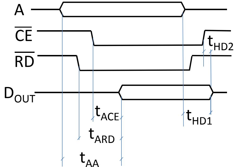
$t_{HD1}$  - hold data time after decaying A
