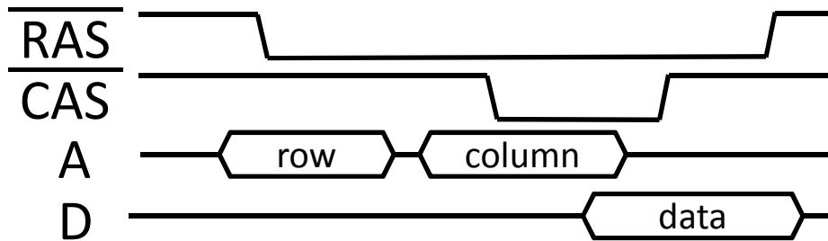
Static columns change of addr. automatically detected, no CAS sync.
