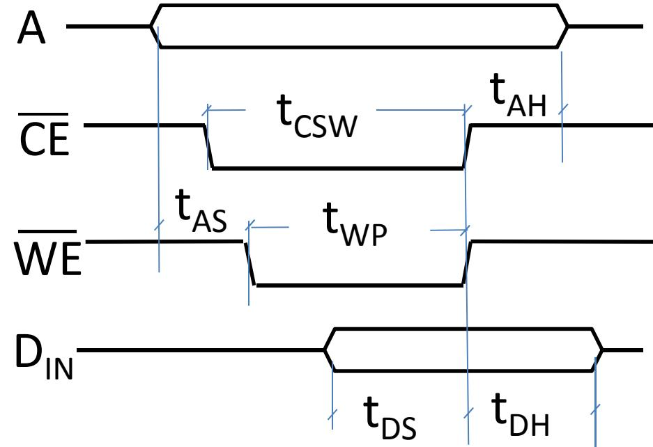
$t_{AS}$  – address setup
